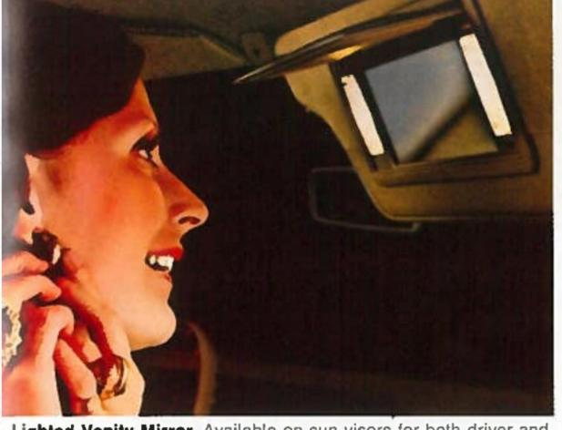
Lighted Vanity Mirror. Available on sun visors for both driver and passenger sides (passenger side only on Convertible). Raising the maintain a selected speed without using the ac- protective cover turns on lamps, one on each side of the mirror. Selector switch for high- or low-intensity light. Tilted, makes an excellent map light. Right-hand version is standard on Talisman.
