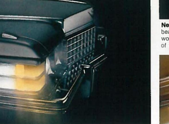
Cornering Lights. For added convenience when driving at night, these lamps project a beam of light from the side of the car to illuminate the roadside and road signs when making a left or right turn. They're located on the side of each front fender and blend beautifully with the front end design of every 1974 Cadillac. The directional turn signal lever will activate them whenever the headlamp switch is on.
