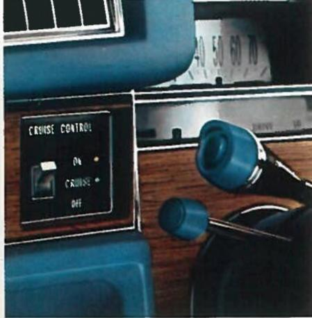
Cruise Control. A touch of this control at the tip of the directional turn signal lever allows you to celerator pedal. Unit automatically disengages when you apply brakes or turn off ignition.
