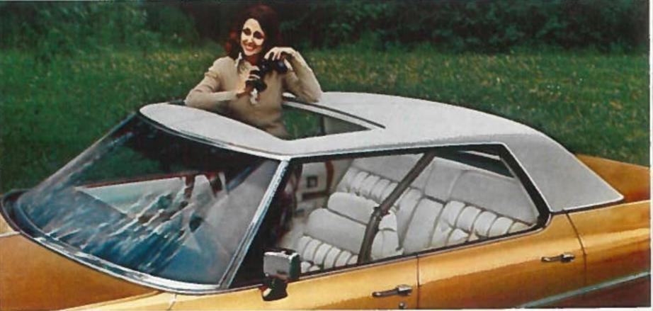
Electrically Operated Sunroof. Simply flick a control switch on the instrument panel, and a roof panel Tilt and Telescope Wheel. This adjustable steering wheel can be slides open overhead to let in the sunshine. It is available on the Fleetwood Brougham, on the Eldorado tilted up or down and moved backward or forward to accommo-Coupe with vinyl roof and DeVilles with vinyl roofs, also Calais when vinyl roof is ordered.
