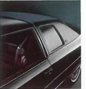
CABRIOLET. This exterior roof design for the Coupe deVille, pictured top right, has a sheer chrome strap, bordered with vinyl welts, that halos the entire backroof section. It is available with or without an electrically operated sunroof.
