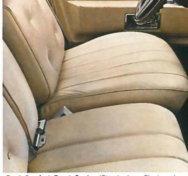
Dual Comfort Front Seats. (Standard on Fleetwood Brougham and available on Eldorado and DeVilles.) One set of seat adjustment controls for the driver's section, and a separate set for the wider passenger section.
