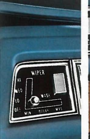
Controlled Cycle Wiper. New for 1974. Adjustable delayed action for light rain (up to 10second intervals between wipes).
