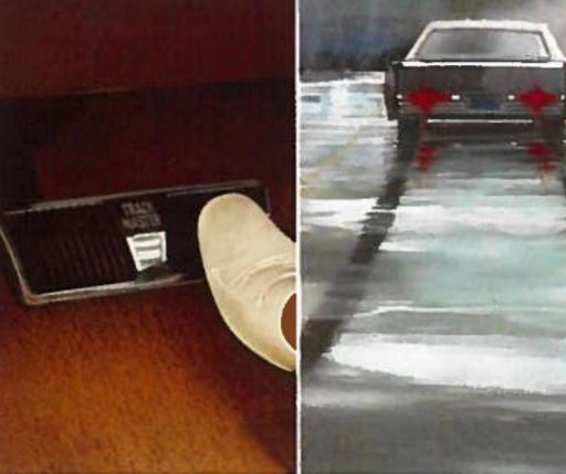
Track Master. This computerized skid-control system automatically pumps your brakes and maintains rear-wheel rotation for improved control during severe braking situations.
