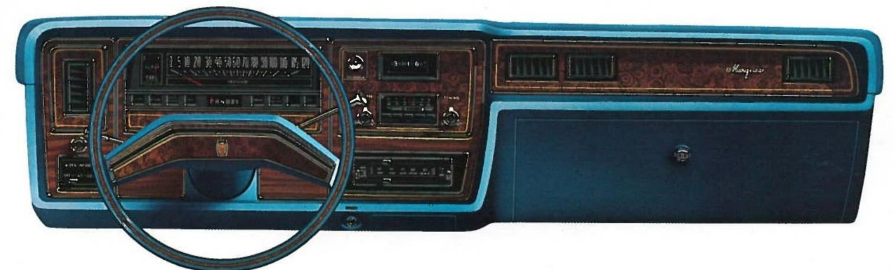
Mercury Grand Marquis instrument panel with optional AM/FM/MPX radio, automatic temperature control, interval windshield wipers and right-hand remote control mirror.
