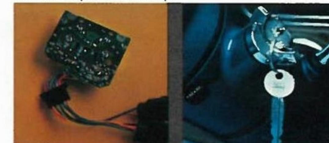
Solid-state ignition doesn't require breaker point replacement
