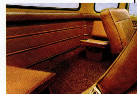
2. Jump seats (optional) have foam-padded cushion and back, fold out of the way quickly when not in use to clear the floor.
